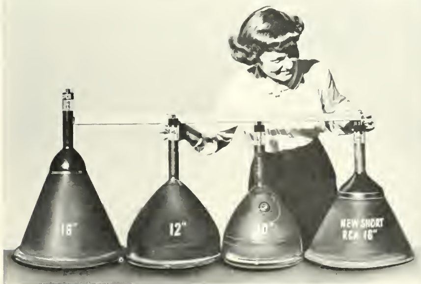
DEVELOPMENT OF THE 16-INCH METAL-CONE KINESCOPE ENABLED SUBSTANTIAL REDUCTION IN THE COST OF LARGE-SCREEN, DIRECT-VIEW TELEVISION RECEIVERS.
